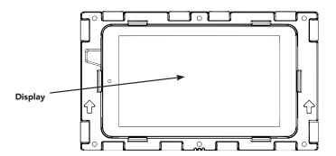
3. Mount the enclosure to the wall using the screw holes in the enclosure. Insert the wall anchors prior to securing the screws in place.
