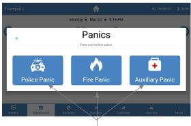
Hold for three seconds to trigger police, fire, OR auxiliary alarm
