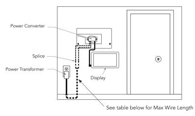
4. Pull wire from touchpad to AC outlet. If replacing an existing touchpad, existing wiring can be used; however, new touchpad must be powered by supplied 12V DC power transformer. Do not power from existing panel.
