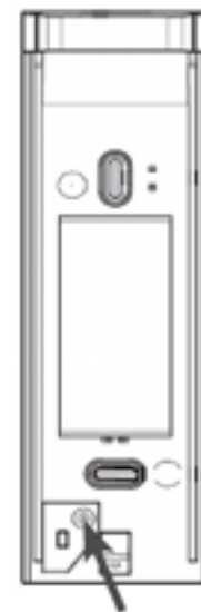
Wall Tamper Hole
